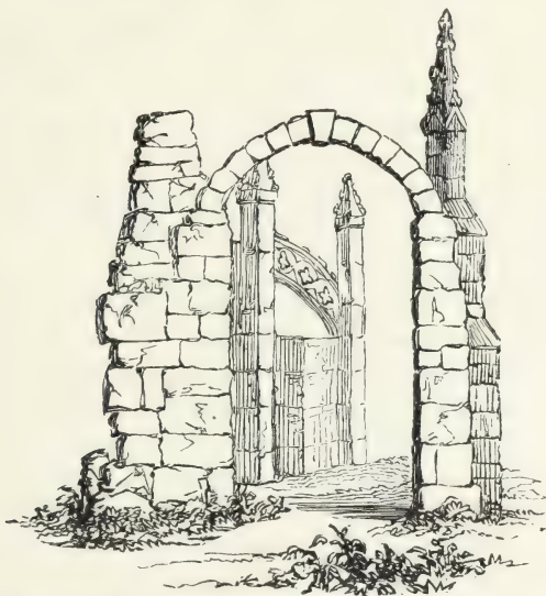
[Fig. 133. Sketch exhibiting the principle of forming abutments for Gothic arches, as generally adopted in ecclesiastical buildings.]
